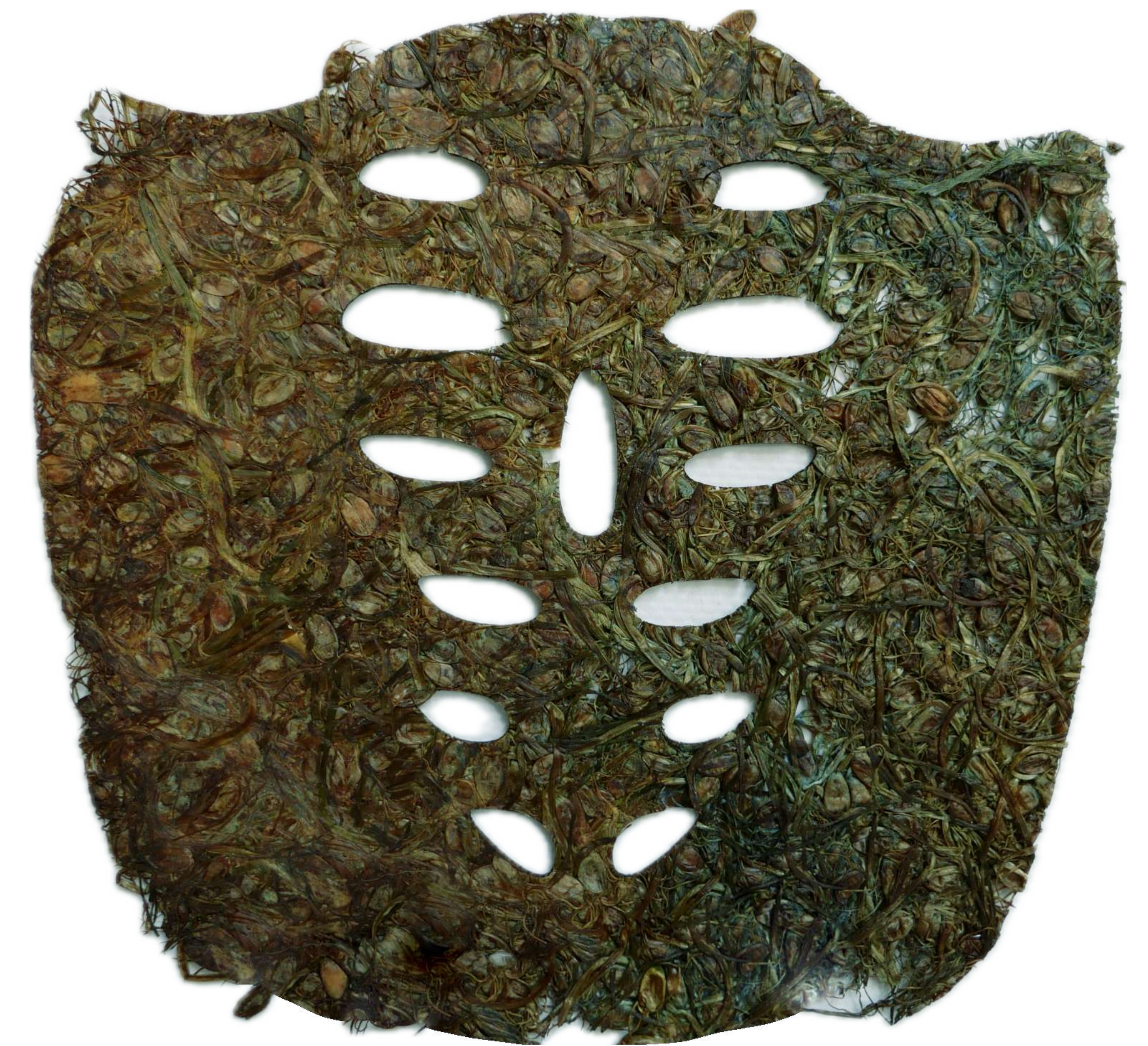
Heat-pressed sample, laser cut patterns, sodium alginate coating & indigo dye
