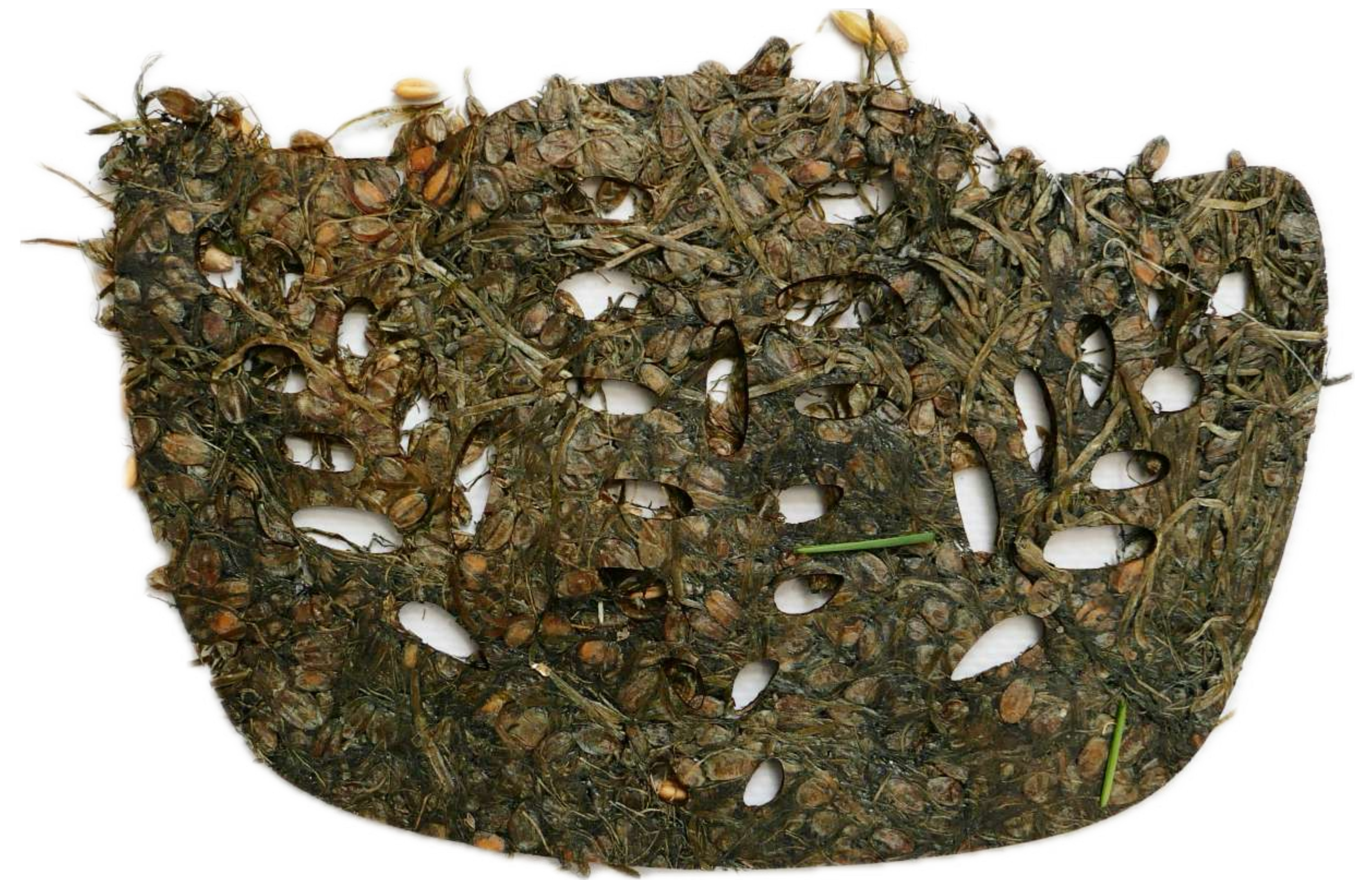
Heat-pressed sample, laser cut patterns, sodium alginate coating & indigo dye
