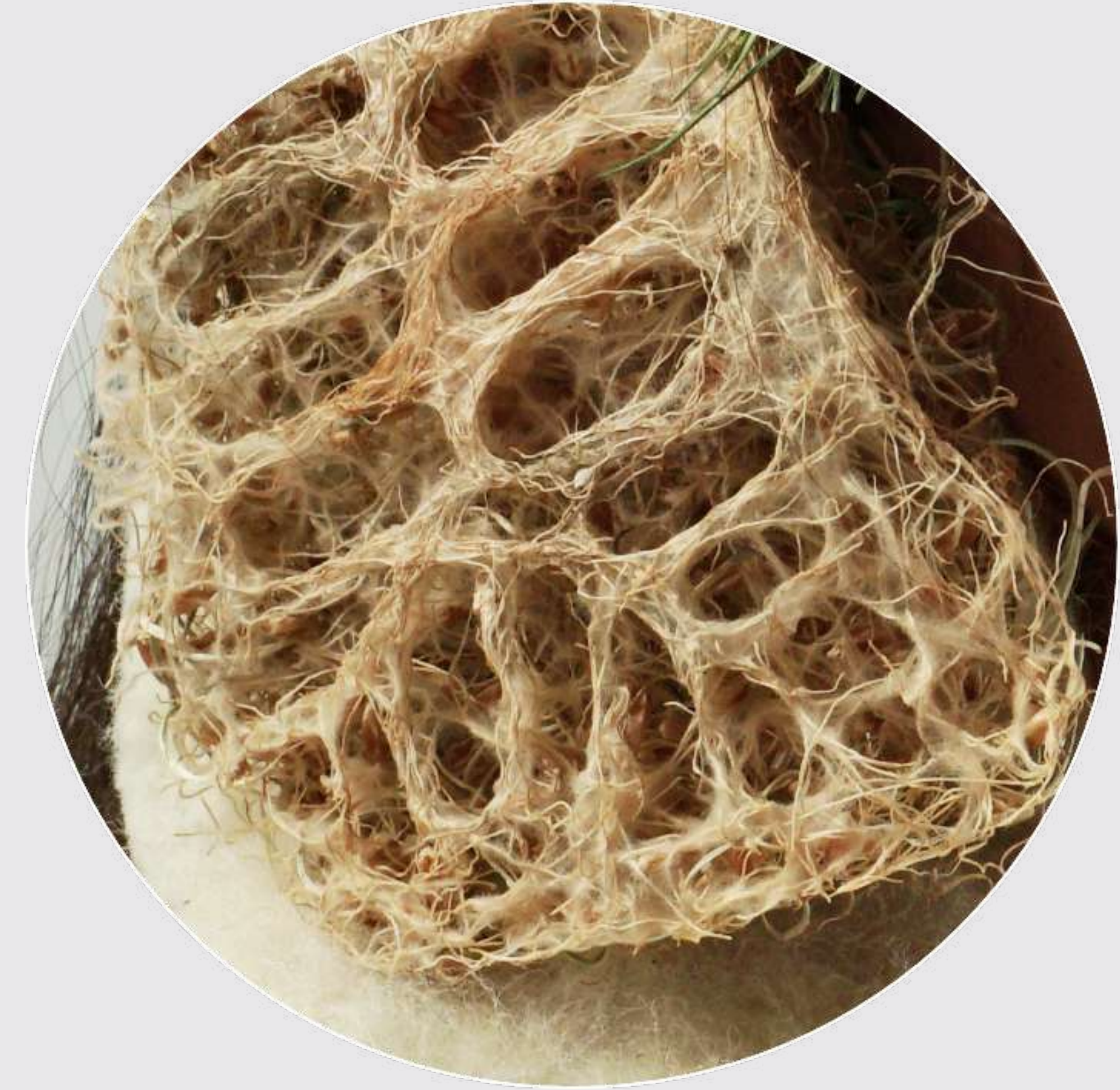
Cultivated wheatgrass structure in 3D printed mould
