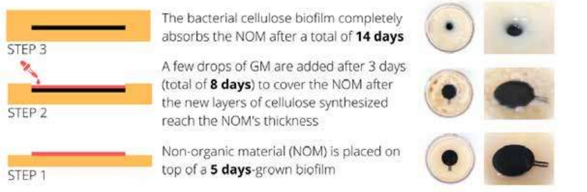
Figure 5: Non-organic materials (NOM) can be embedded in 3 steps by taking advantage of bioassembling. We illustrate this here with a large conductive pad (3cm) that was 3D-printed using Protopasta carbon-based conductive PLA filament. ©Madalina Nicolae & Vivien Roussel
